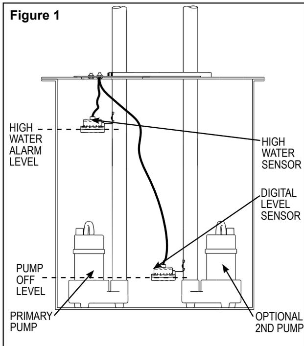
water sensor, the controller will cue audible, visual, and any remote alarms indicating a high water level.
